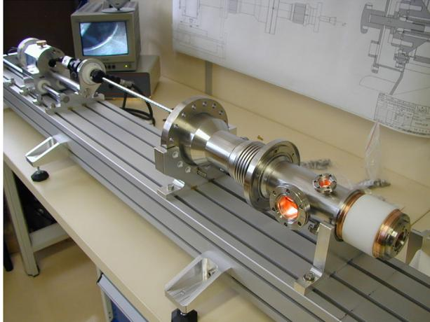
Figure 7: Reception test of a TTF-III Coupler.
