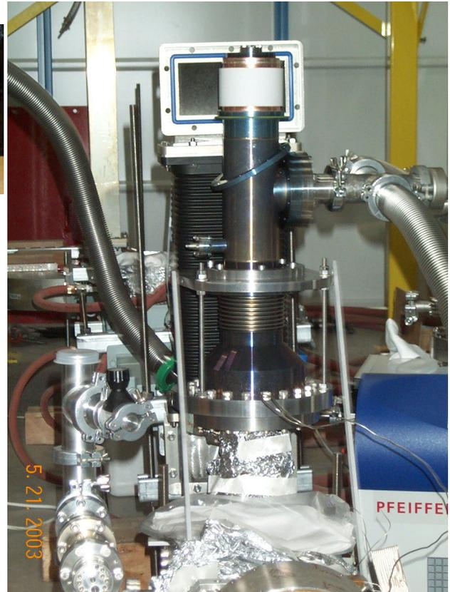
Figure 6: TTF-IV coupler being assembled on the high power test bench.
