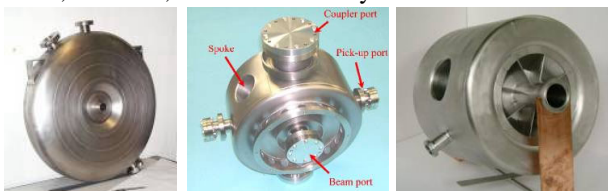
Figure 3: 352 MHz cavities. From left: \beta > 0.1 reentrant (LNL) [12], \beta = 0.2 Spoke (LANL) [13], and \beta = 0.35 Spoke (IPNO) [14].
