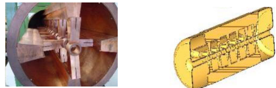
Figure 5: \beta=0.1 CH structures under development at the University of Frankfurt: (left) model of the 352 MHz, 19-gap [17] and (right) sketch of the 174 MHz, 16-gap [18] resonators.
