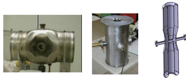
Figure 6: Half wave resonators. From left: \beta=0.28 , 322 MHz (MSU) [19]; \beta=0.31 , 352 MHz (LNL) [20]; \beta=0.12 , 160 MHz (KFZ Juelich) [21].
