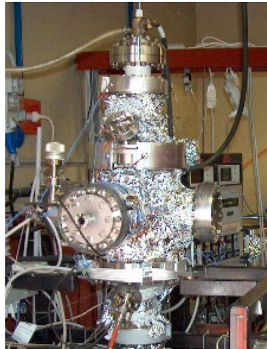
Figure 9: Picture showing the UHV linear arc system mounted in “Tor Vergata” University. The 200mm central chamber allows an easy mounting of samples to check quality and uniformity of the niobium deposited film.
