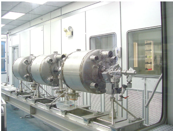
Figure 1: Medium Beta Cavity String in clean room.
