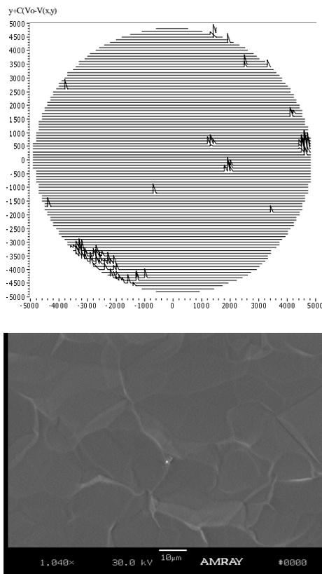
Figure 3: FE scan result from the witness sample for combined HPR, evacuation and vertical RF test process on SNS cavity MB21. Also shown is an electron microscopic picture of an emitter which contains Nb, Ag, Cu, Ti.
