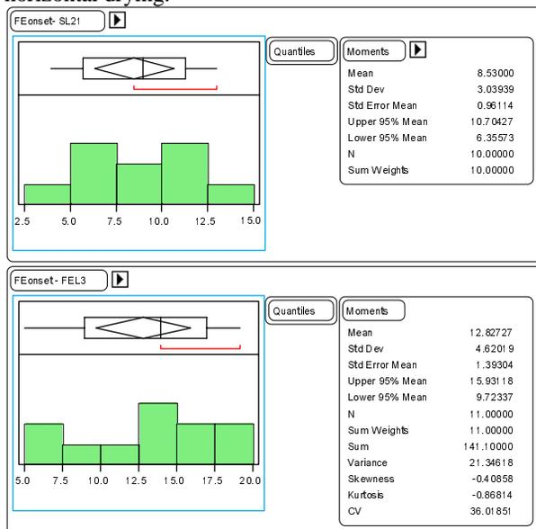
Figure 5: Performance comparison of FEL3 and SL21 cavities.
