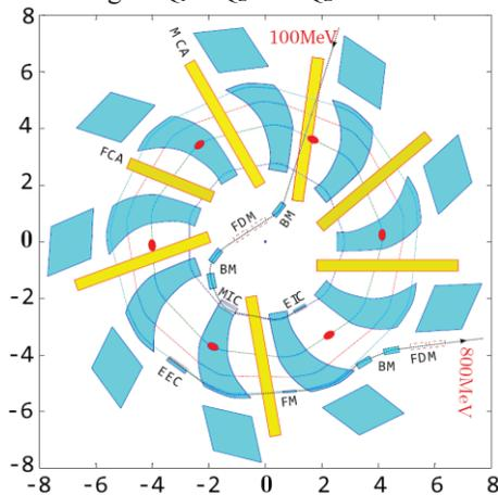
Figure 7: The latest layout sketch of the 800 MeV cyclotron solution, including injection and extraction elements (MCA: main cavity, FCA: flat-top cavity, FDM: focusing doublet, BM: bending magnet, MIC: magnetic injection channel, EIC: electric injection channel, FM: focusing magnet, EEC: electric extraction channel).
