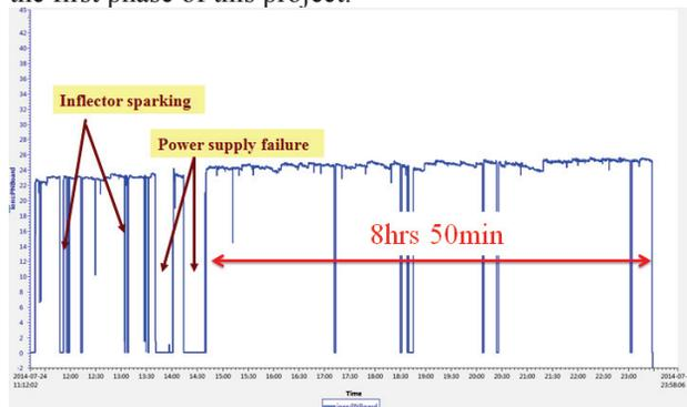
Figure 5: Beam current history during 12 hours continuous operation.
