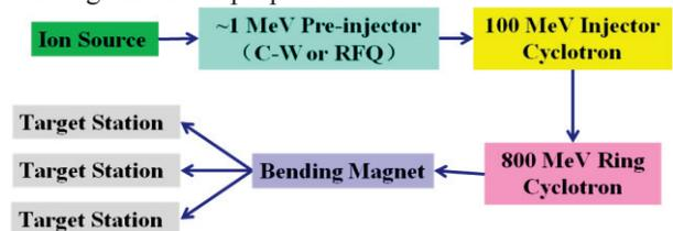
Figure 6: The block diagram of the proposed high power cyclotron complex.
