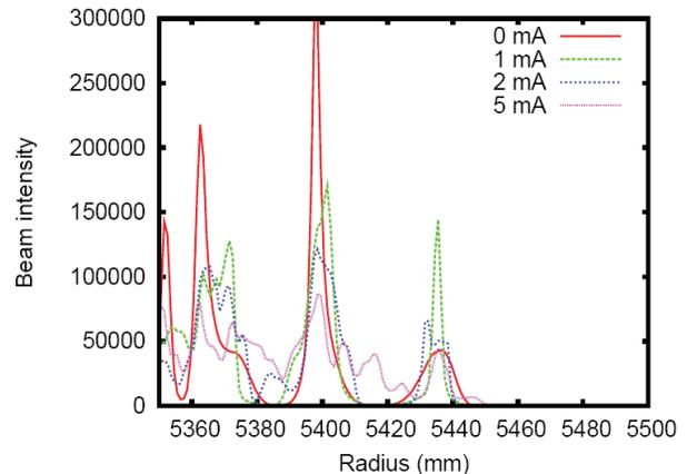
Figure 9: Radial beam profile of the last few turns for different beam current scenarios.
