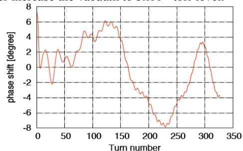
Figure 2: The integral phase slip of the final field map.
