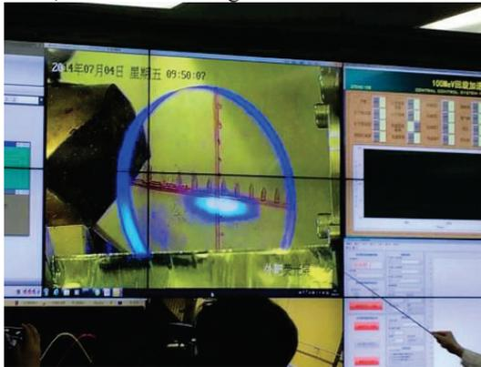
Figure 4: The quartz plate diffuses blue light when it is penetrated by the 100 MeV proton beam.
