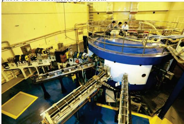
Figure 1: Photo of the assembled 100MeV compact cyclotron.
