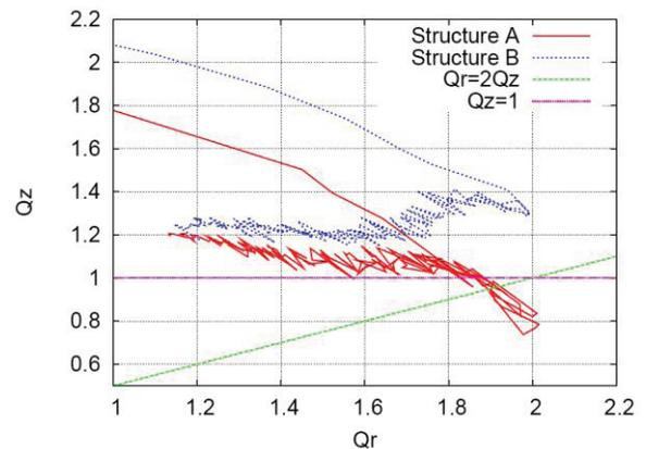
Figure 8: Tune diagram of the structure A (last version) and structure B (current version).
