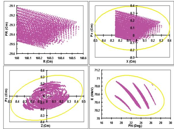
Figure 3: The total extracted beam distribution on the stripping foil. The yellow lines are the phase space boundary with 5 time realistic emittance.
