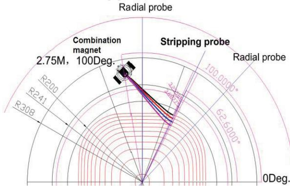
Figure 1: Positions of stripping points for extracted energy of 70MeV, 80MeV, 90MeV and 100MeV.
