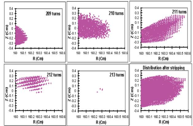
Figure 2: The extracted particle distribution for each turn.
