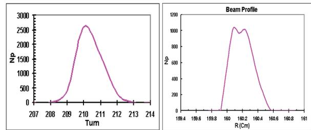
Figure 4: The extracted particle distribution and extracted beam profile on the stripping foil.
