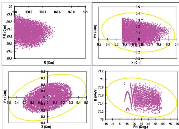
Figure 7: The total extracted beam distribution on the stripping foil. The yellow lines are the phase space boundary with 5 time realistic emittance.
