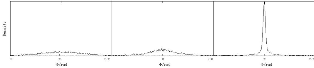
Figure 5 : Beam density evolution during the bunch compression in CSRm. The initial density of the heavy ions (left), the density at a fixed time during the bunch compression(middle), and the density at 1/4 synchrotron period(right).
