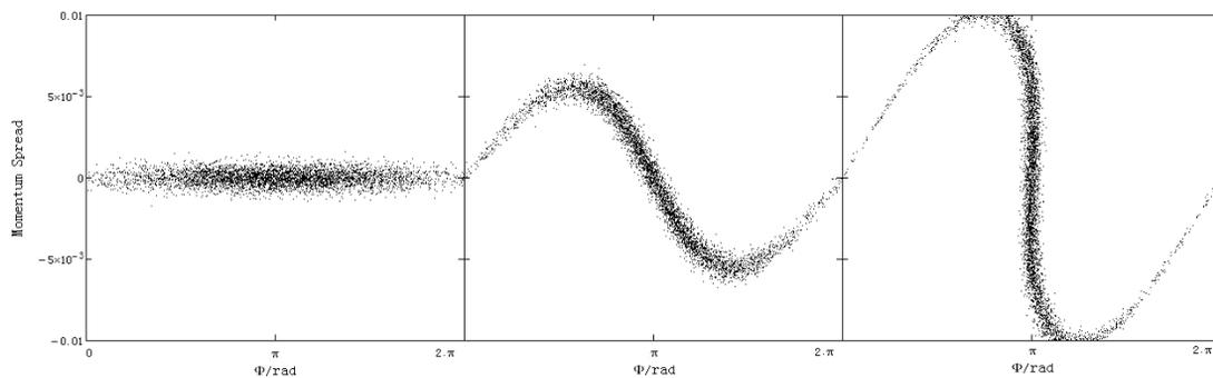
Figure 4: Phase space evolution during the bunch compression in CSRm. The initial phase space distribution(left), phase space distribution at a fixed time during the bunch compression(middle), and the phase space distribution at 1/4 synchrotron period(right).
