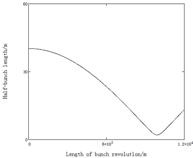
Figure 1: Half bunch length as a function of revolution length during bunch compression in CSRm.
