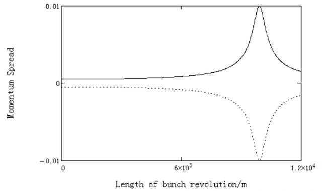
Figure 3: Momentum spread at mid-pulse as a function of revolution length during bunch compression in CSRm.
