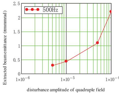
Figure 4: Extracted beam horizontal emittance vs. quadrupole field disturbances amplitude.
