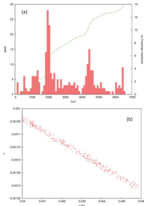
Figure 3: Extracted spill intensity vs. revolution turn (a) and distribution in horizontal phase space (b) under  $1\cdot 10^{-5}$  quadruple field disturbances.
