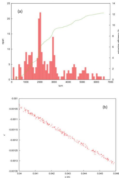
Figure 5: Extracted spill intensity vs. revolution turn (a) and distribution in horizontal phase space (b) under  $2 \cdot 10^{-5}$  dipole field disturbance at 500 Hz
