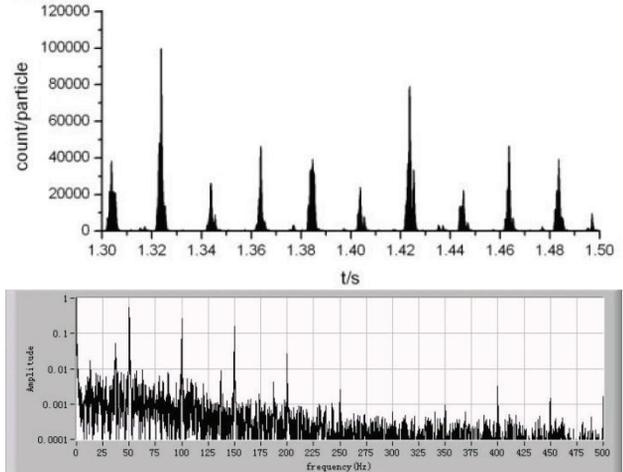
Figure 1: Extracted beam spill intensity variation in time domain and frequency domain [2,3].
