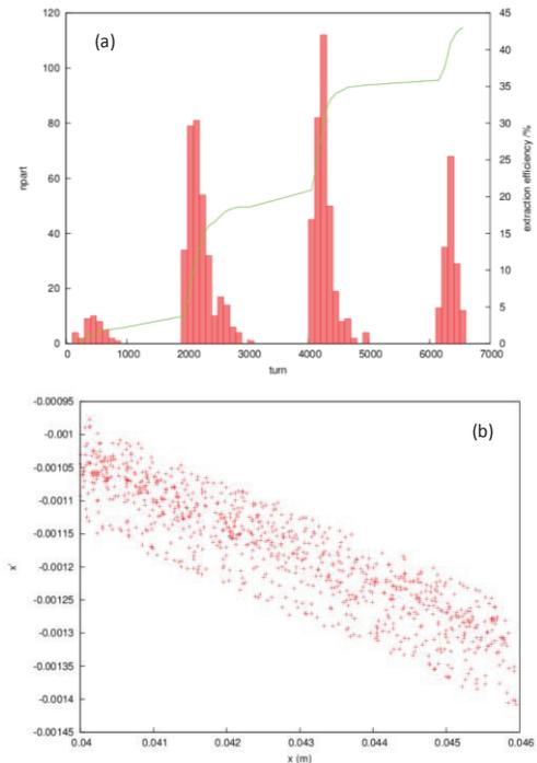
Figure 2: Extracted beam spill intensity vs. revolution turn (a) and distribution in horizontal phase space (b) under  $1\cdot 10^{-4}$  quadruple field disturbances.
