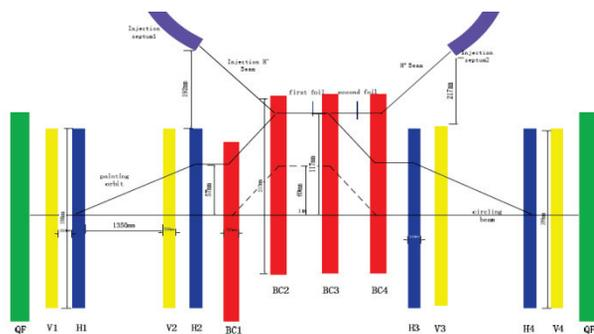
Figure 1: Injection component layout. BC1~BC4: Fixed orbit bump magnets, BH1~BH4: horizontal painting bumpers, BV1~BV4: vertical painting bumpers, ISEP1&2: septum.
