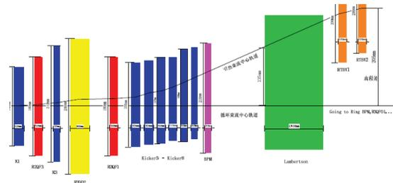
Figure 5: The layout of final extraction scheme.
