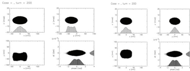
Figure 3: Beam distribution in phase spaces at injection end by an x-y correlated(left) and anti-correlated(right) phase space painting.
