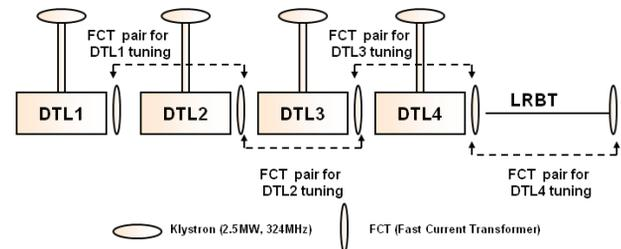
Figure 3: The RF driving and FCT on linac.
