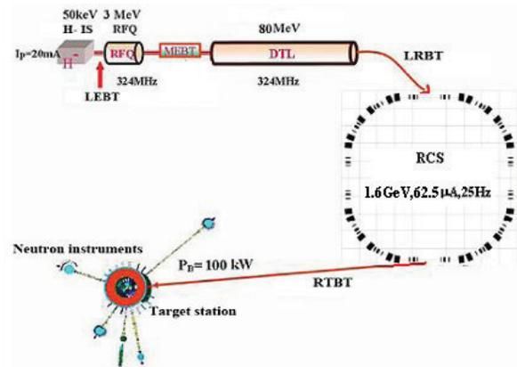
Figure 1: The schematic layout of CSNS.
