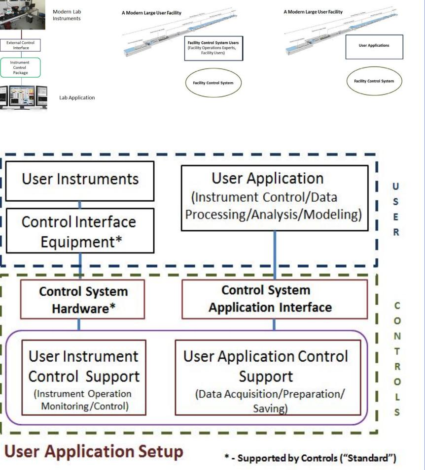
The DCTS control system software, which manages instrument operational functions based on the control hardware, forms a user instrument control support package.
