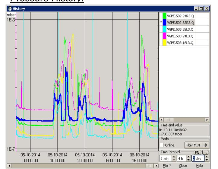
The pumping group pressure gauges history is an additional tool to check pumps efficiency, analyse pumping speed and detect leaks.
