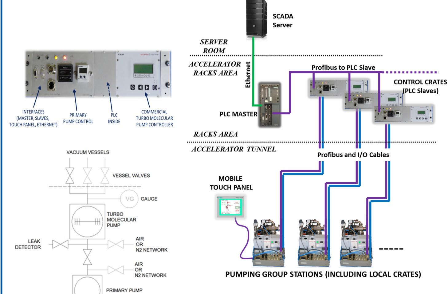
Transitions between modes are requested either by the operator or by the process itself. Phase sequencer, including series of steps with transition conditions and time dependencies, sends "AUTOMATIC" orders to devices of pumping group in order to reach final state of group, depending on mode. "Pump" mode Sequencer:
