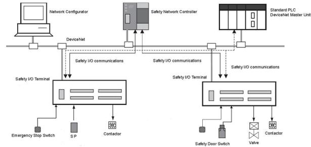
Figure 2: DeviceNet schematic.
