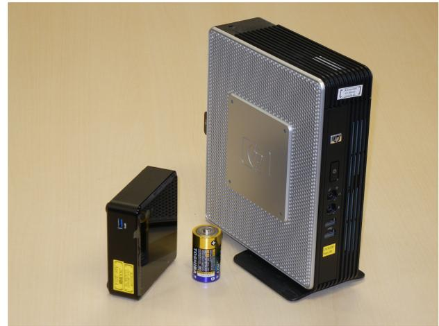
Figure 1: Photograph of HP Compaq t5730 (left), Intel NUC (right), and a D Battery for Size Comparison (center). T5720 is not shown but its appearance is almost same as t5730.
