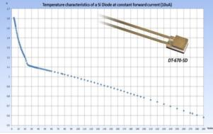
Figure 3: Diode sensor DT 670-SD characteristic curve [5].
