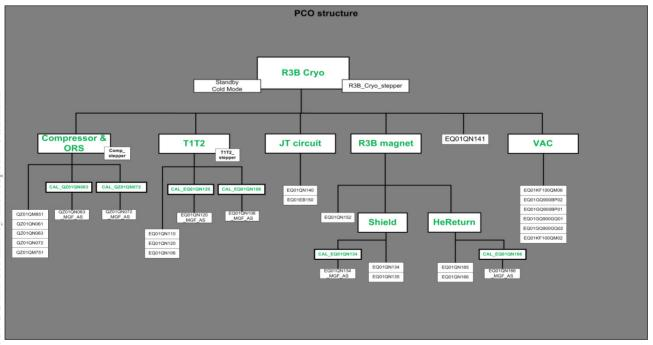
Figure 1: UNICOS unit (PCO) structure of the R<sup>3</sup>B facility.
