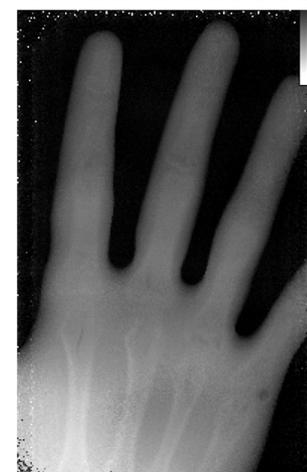
Proton radiographs of head (left) and hand phantoms (right).
