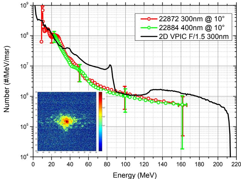
Proton spectra from interaction of LANL Trident laser with 80J, 600fs,  $r < 2\mu\text{m}$  with 300nm and 400nm  $\text{CH}_2$  targets. Inset shows focal spot with F/1.5 off-axis parabola.
