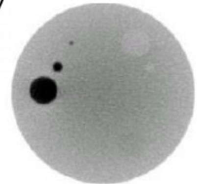
Reconstructed images based on GEANT4-simulated 200 MeV pCT data of the illustrated phantom.
