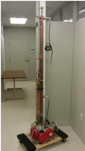
Multiharmonic buncher F=40.25, 80.5, 120.75 MHz P\sim 100 W total
