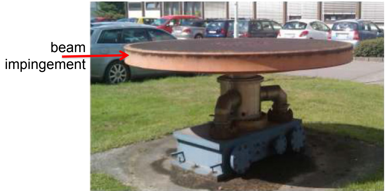
Prototype of a rotating tungsten target from the German SNQ project, ca. 1985.
