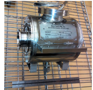
Solenoid installed in He vessel
