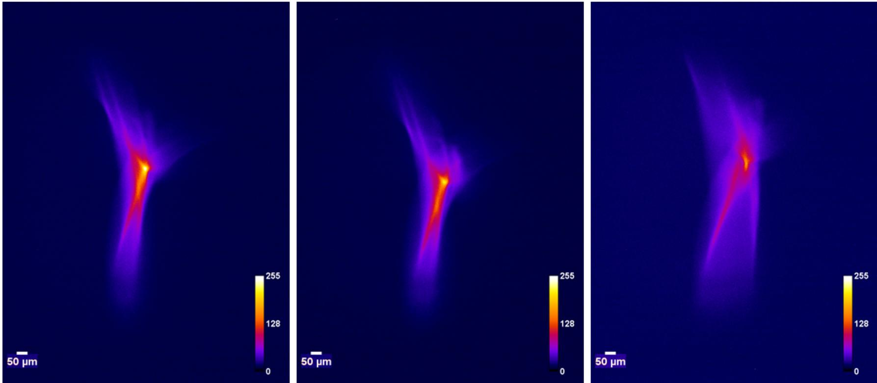
↑ 1<sup>st</sup> beam images taken in late July at Pegasus: 1.2 pC single bunch and wide FOV setup, 50 mm camera lens and 3.75x magnification. Even at this low magnification, ~ 10 μm features are evident in the beam. Spot sizes smallest achievable during recent Pegasus beamline re-commissioning.
