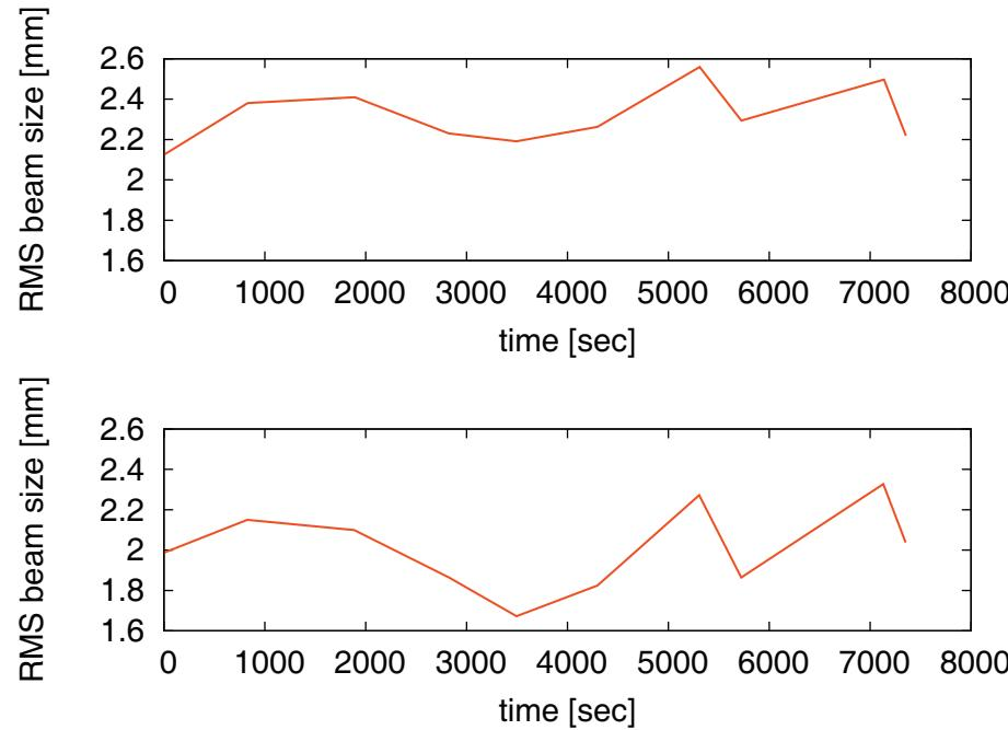
RMS beam size remains unchanged regardless of mis-steering and tunemeter blow-up efforts - independent of intensity
