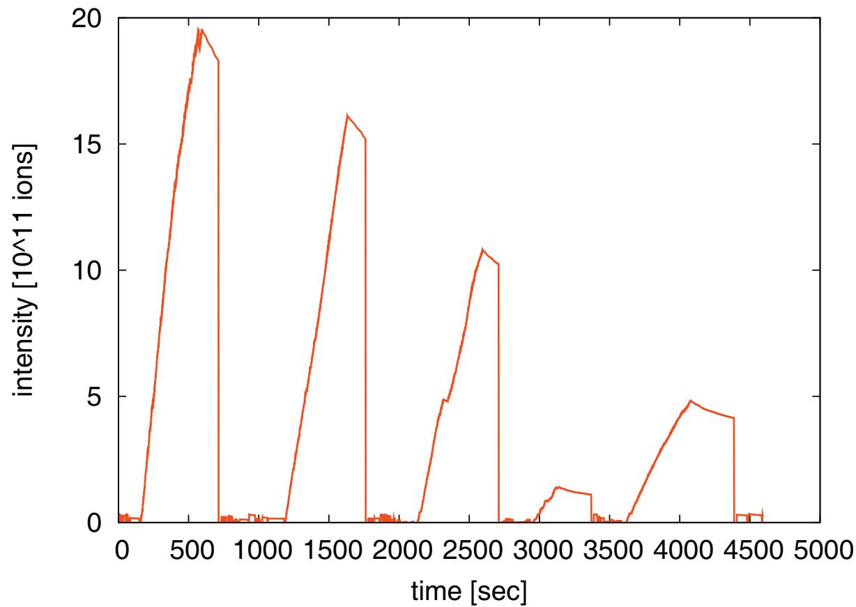
Reduced injection efficiency due to mis-steering
