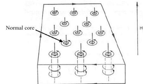
If vortices penetrate at  $B_{c1}$ , all alternative SRF materials would be severely limited.
