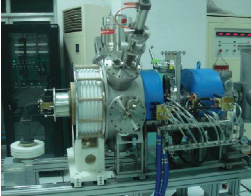
A 60mA/50 keV ECR ion source has been set up.
