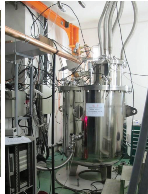
A cryostat at 4K for horizontal test of spoke cavity has been set up .
