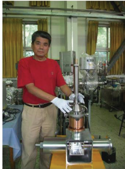
162.5MHz, HWR CW, 20kW Tested
