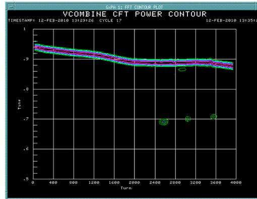
Evolution of V and H. tune monitored over time for intensities from 2 to 15 injected turns
