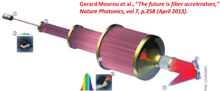
Figure 2: Principle of a coherent amplifier network (CAN) based on fiber laser technology. An initial pulse from a seed laser (1) is stretched (2), and split into many fibre channels (3). Each channel is amplified in several stages, with the final stages producing pulses of ~1 mJ at a high repetition rate (4). All the channels are combined coherently, compressed (5) and focused (6) to produce a pulse with an energy of >10 J at a repetition rate of 10 kHz (7). [3]
