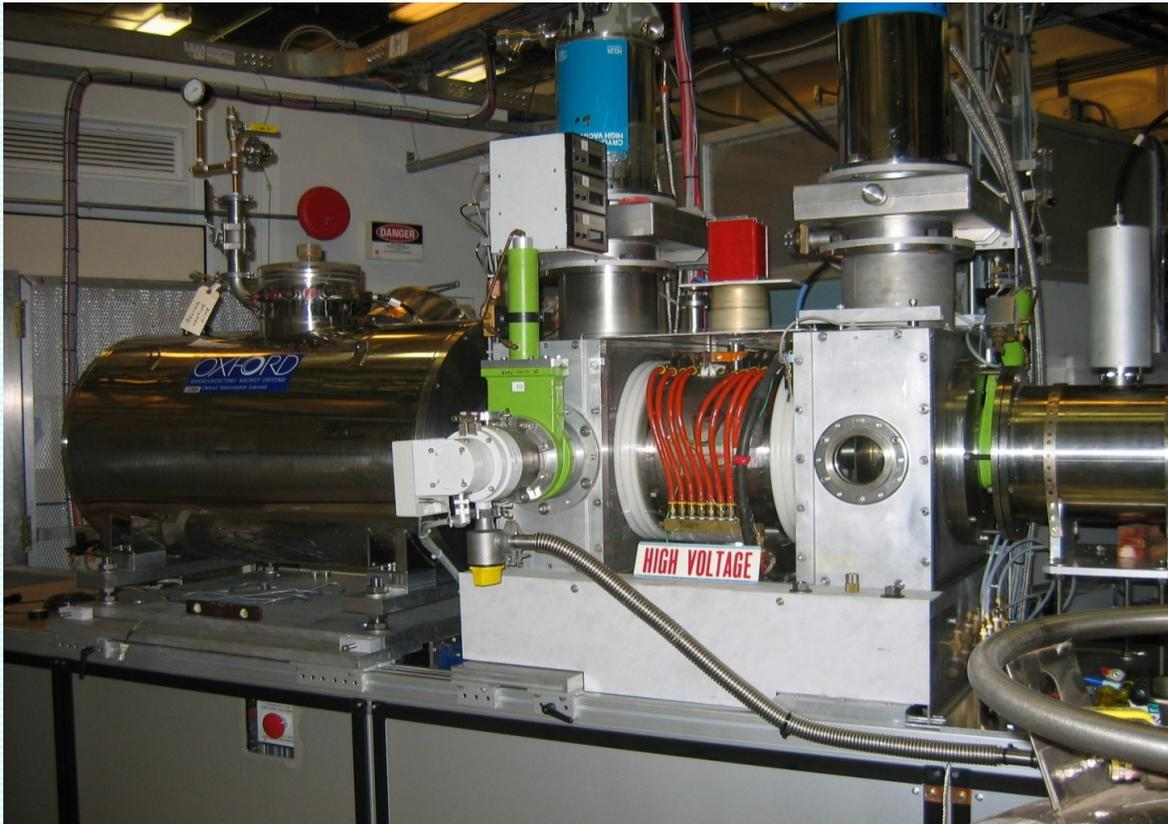
RHIC OPPIS produces reliably 0.5-1.0mA polarized H<sup>-</sup> ion current. Polarization at 200 MeV: P = 80%.
