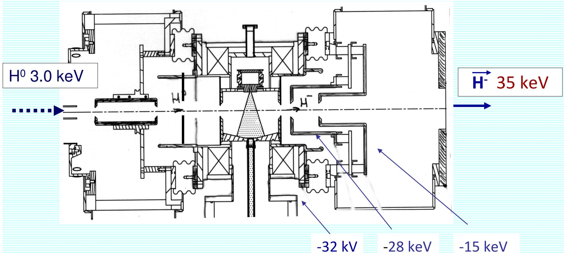
Na-jet cell is isolated and biased to  $-32$  keV. The H<sup>-</sup> beam is accelerated in a two-stage acceleration system.
