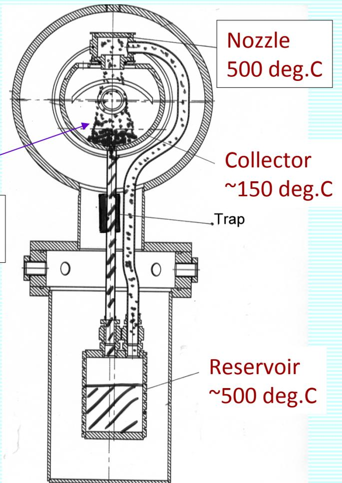
Reservoir– operational temperature.  $T_{res.} \sim 500$  °C.
