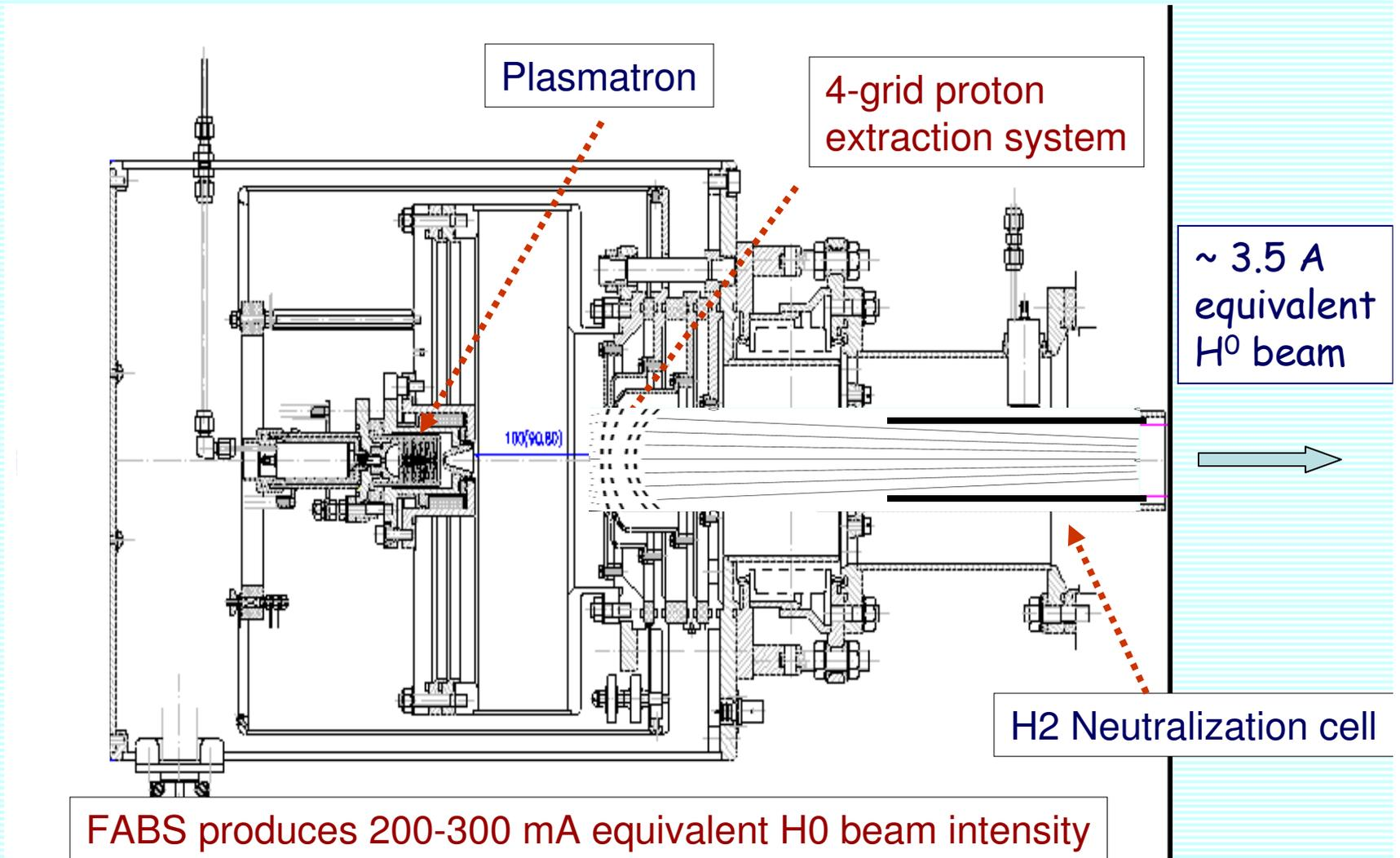
FABS produces 200-300 mA equivalent H<sup>0</sup> beam intensity
