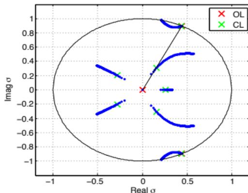
From the controller, the system is sampled at  $T_{rev}$ . Plots shows the eigenvalues of the system  $\lambda_i$  in Z-domain ( $z_i = e^{\lambda_i T_{rev}}$ ) for increasing gain  $G$ .
