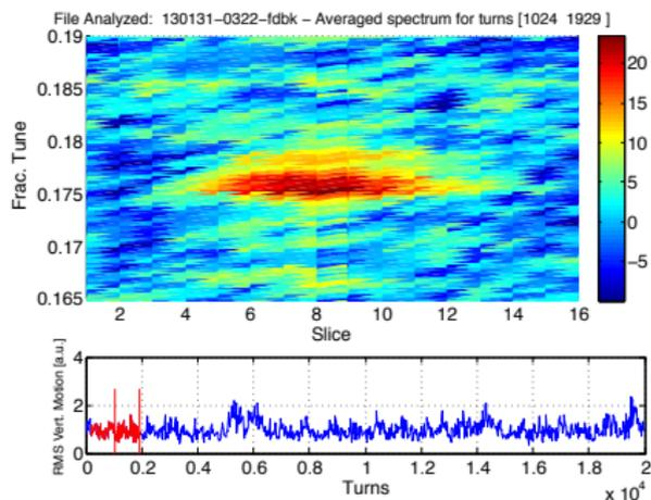
Open loop - Spectrogram for multiple samples across the bunch for turns 0-2000
