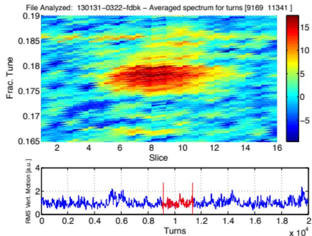
Closed loop - Spectrogram for multiple samples across the bunch for turns 9K-11K
