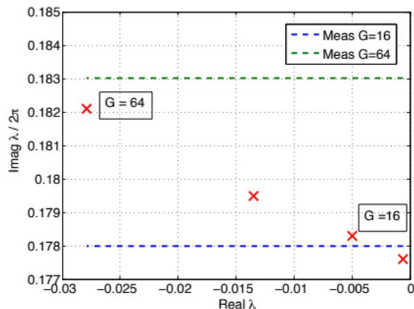
Dominant eigenvalues of the feedback system for  $G = 8, 16, 32, 64$ . Comparison with frac. tunes measured for  $G = 16, 64$  phase  $\phi = 30^\circ$
