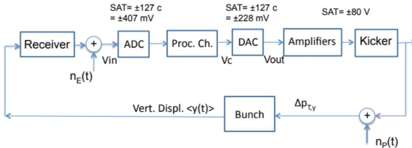
4 GS/sec. digital channel. Flexible reconfigurable processing - 2 ADCs / 1 DAC
