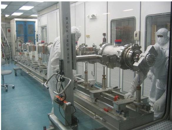
Figure 4: Cavity string assembly in Class 100 cleanroom.
