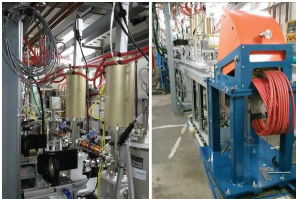
Figure 8: Phase I diagnostics systems in the BTF. Left: the 2-slit emittance meter. Right: the spectrometer dipole.
