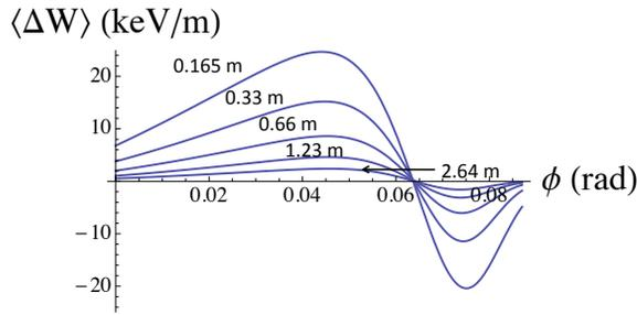
Figure 1: Approximate expression (8) for the difference in mean energy loss with and without the effect of upstream bends for a linearly compressing Gaussian bunch propagating through Bend 3 of the chicane of Table 1. The result is shown for various values of the central drift length.
