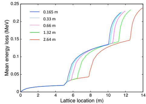
Figure 3: The cumulative loss in the mean energy of the bunch along the length of the chicane is shown for the values  $L_c = 2.64$  m, 1.32 m, 0.66 m, 0.33 m, and 0.165 m.
