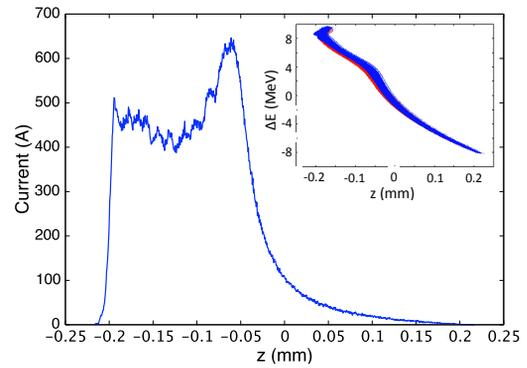
Figure 2: Current profile at the exit of BC2. The head of the bunch appears on the left ( $z < 0$ ). (Inset) Longitudinal phase space at the exit of BC2 with (blue) and without (red) the effects of longitudinal CSR included.
