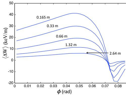
Figure 4: Difference between the longitudinal CSR wakefield in Bend 3 of BC2 as computed using the model of [2] (without upstream transient effects) and [3] (with upstream transient effects) during IMPACT-Z simulation. The average of this quantity over the length of the bunch is shown as a function of bend entry angle. Compare Fig. 1.
