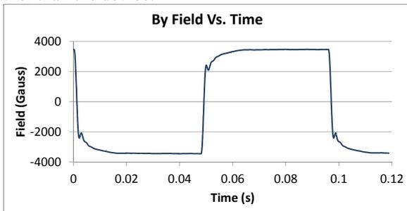
Figure 3: Time-dependence measurement of a one-period test model. The vertical field was  $\pm 3500$  Gauss, switched at 10 Hz.
