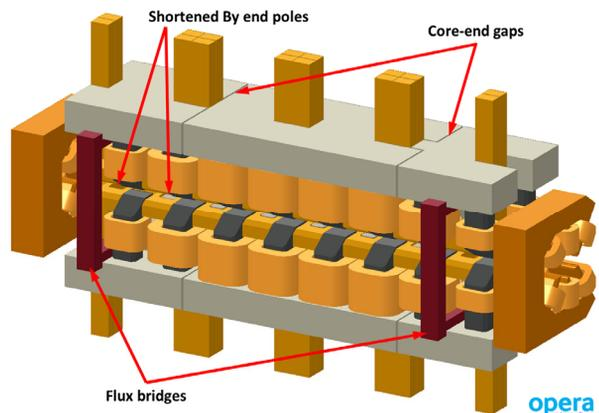
Figure 5: Magnetic field analysis model of the four-period test model.
