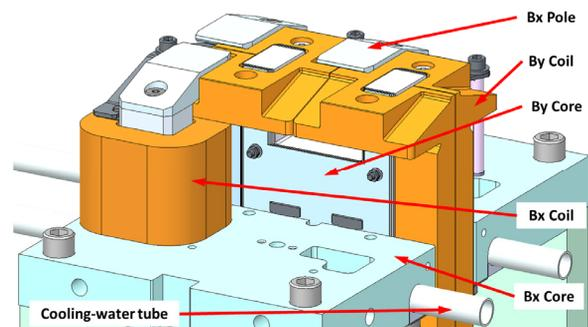
Figure 1: A 3-D CAD model of the one-period test model lower jaw (one  $B_x$  coil/pole assembly is hidden to show the  $B_y$  core).
