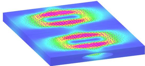
Figure 7: Simulated eddy currents in an aluminum vacuum chamber.
