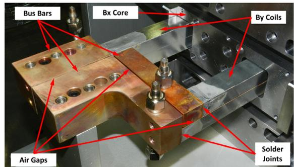
Figure 4: Solder joints of the By coils to the bus bars.
