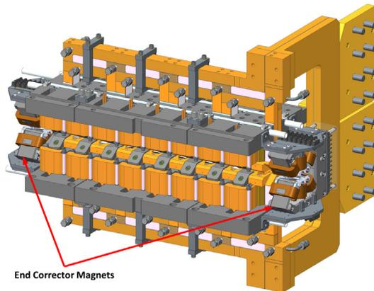
Figure 6: A 3-D CAD model of the four-period test model.
