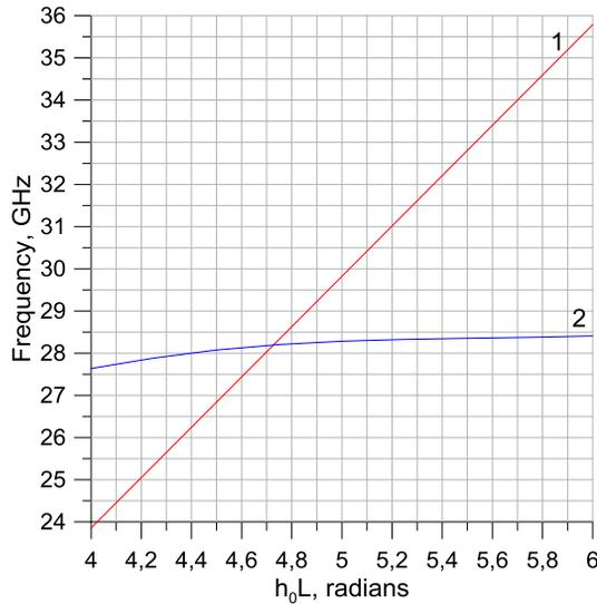
Figure 1: Dispersion characteristics: 1 – light cone line, 2–dispersion curve of  $TM_{01}$ - $TM_{11}$  wave in HSFC structure.
