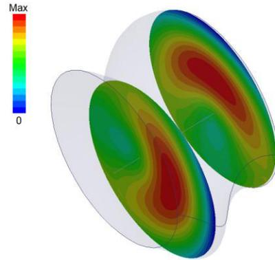
Figure 3: Module of electric field in two sequent cross-sections.
