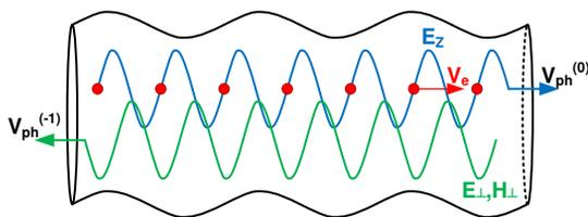
Figure 6: RF undulator excited by bunches itself.
