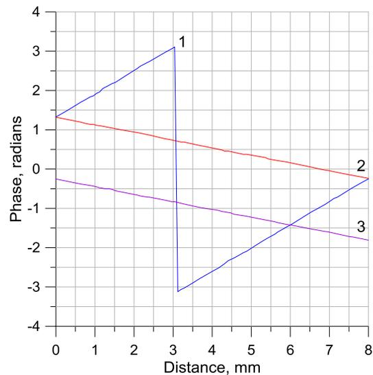
Figure 4: Phases of  $E_z$  (longitudinal) field component (curve 1) and phases of  $E_x$  (curve 2) and  $E_y$  (curve 3) field components.
