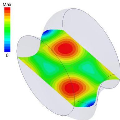
Figure 2: Module of electric field in middle plane.
