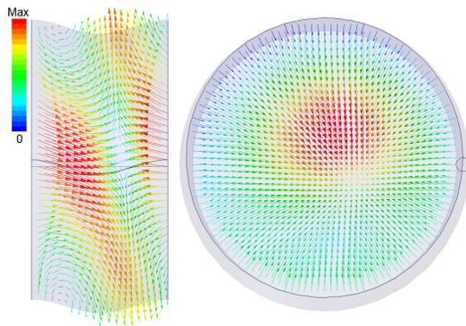
Figure 6: Instantaneous field structure of  $TM_{01}$ - $TM_{11}$  operating wave at phase 190 degrees.
