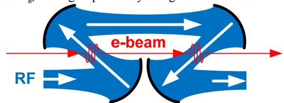
Figure 1: Mirror transfer line employing the “flying” RF undulator.
