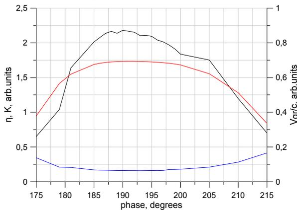
Figure 5: Normalized characteristics of  $TM_{01}$ - $TM_{11}$  wave. The blue curve is undulator parameter. The red curve describes group velocity. The black curve is gain factor.
