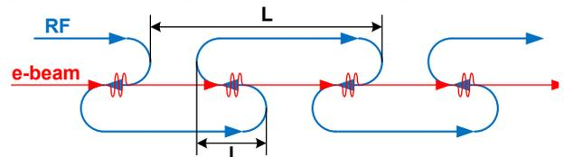
Figure 2: Equivalent scheme of “flying” RF undulator.
