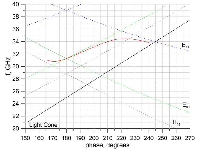
Figure 4: Dispersion characteristic of normal  $TM_{01}$ - $TM_{11}$  wave in helical waveguide (red curve).
