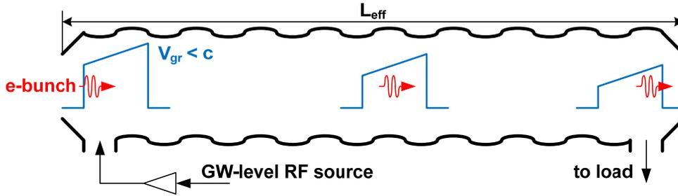
Figure 3: “Flying” RF undulator in form of helical corrugated waveguide section.
