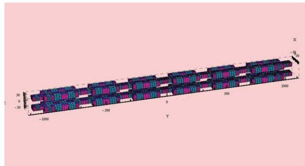
Figure 1: RADIA model of magnet structure for a Knot undulator.
