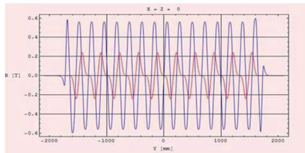
Figure 2: Field distribution of Knot undulator.
