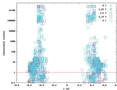
Figure 8: The MP impact location in the cavity body. For reference, the extrusion edge of the vacuum port and instrumentation port are at  $X = -0.6$  m and  $0.6$  m, respectively.
