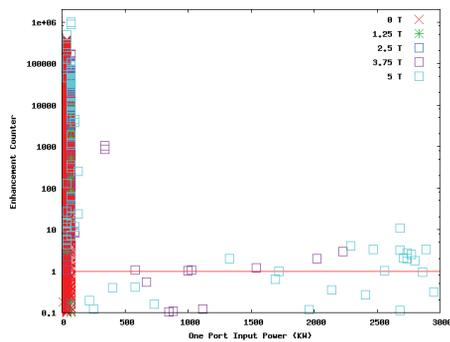
Figure 3: The EC spectrum in the coaxial waveguide.
