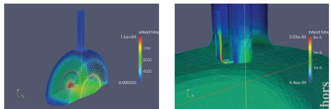
Figure 2: RF field of the cavity. The left figure shows the E field magnitude in the cavity. The right figure shows the maximum B field in the cavity on the coupler loop, where sufficient cooling should be supplied.
