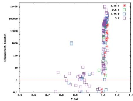
Figure 4: The MP impact location in the coaxial waveguide, where  $Y = 1.1\text{ m}$  is near the RF window.
