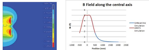
Figure 1: The ANSYS magnetic field calculation of the Lab\_G magnet. The left figure is the contour plot of the field magnitude. The right figure is the comparison of magnetic fields from ANSYS with previous G4Beamline results [5] along the central axis.
