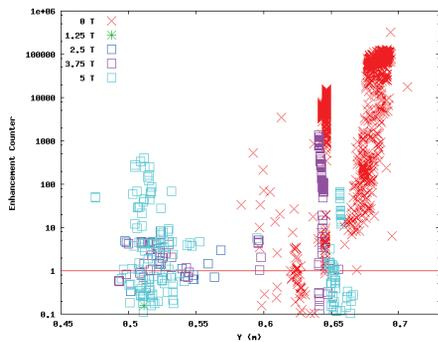
Figure 6: The MP impact location in the coupler. For reference, the extrusion transition between cavity and waveguide is from  $Y = 0.601$  m to  $0.627$  m.
