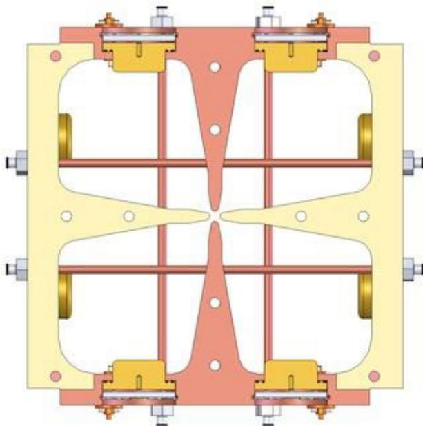
Figure 3: CAD model cross sectional view of the RFQ.
