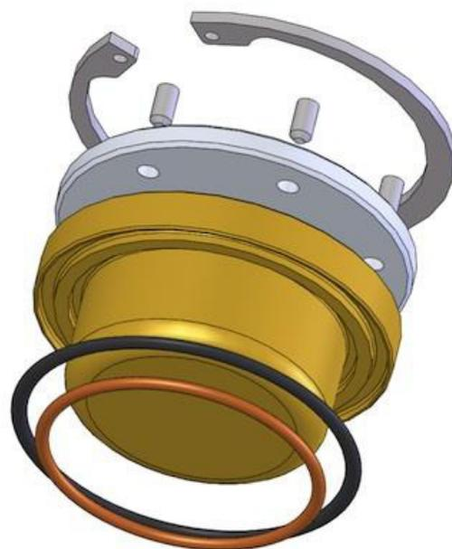
Figure 4: Fixed slug tuner components.
