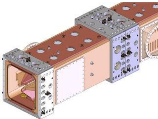
Figure 5: CAD showing a module-to-module joint.
