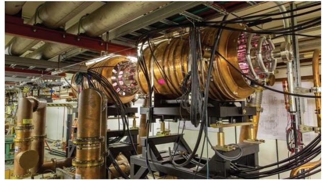
Figure 3: Two complete cavities installed in the Recycler.
