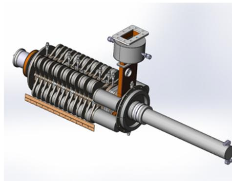
Figure 1: The 10 kW CW S-Band PPM Klystron.
