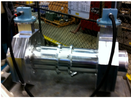
Figure 1: Two wrap-around mode converters for insertion loss measurements of lossy ceramic cylinders. S11 was measured to be less than -23.2 dB at the center frequency.
