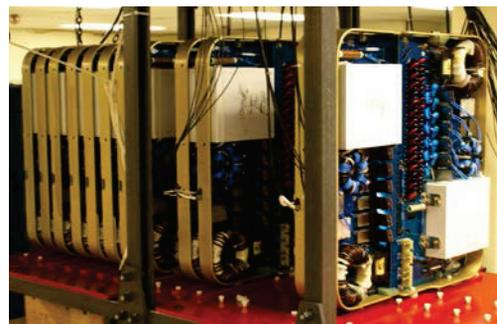
Figure 5 Stack of twenty-four connected modules.
