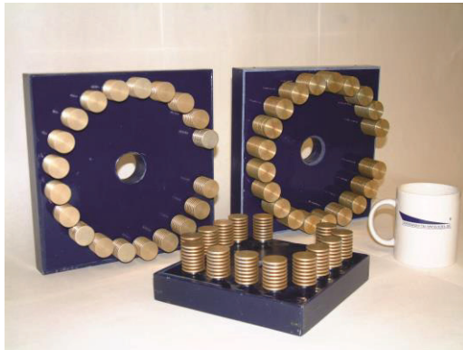
Figure 5: Three DTI 10 kV solid-state switchplates.
