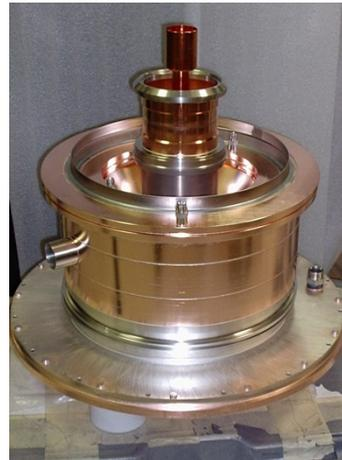
Figure 5: Collector and output window and waveguide assembly.
