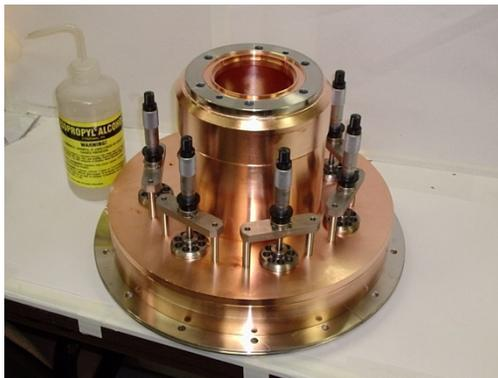
Figure 4: Input cavity assembly.
