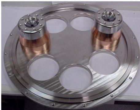
Figure 1: Gun support plate with two guns.
