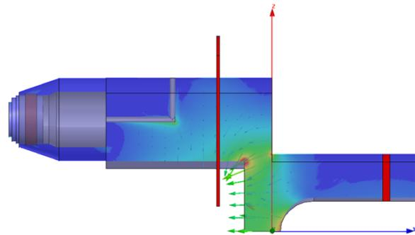
RF field gradient:  $E_{max}=2kV/cm$  with 1kW total input drive
