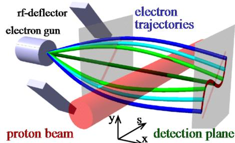
Figure 1: Schematic of an electron scanner for the vertical beam profile [1].
