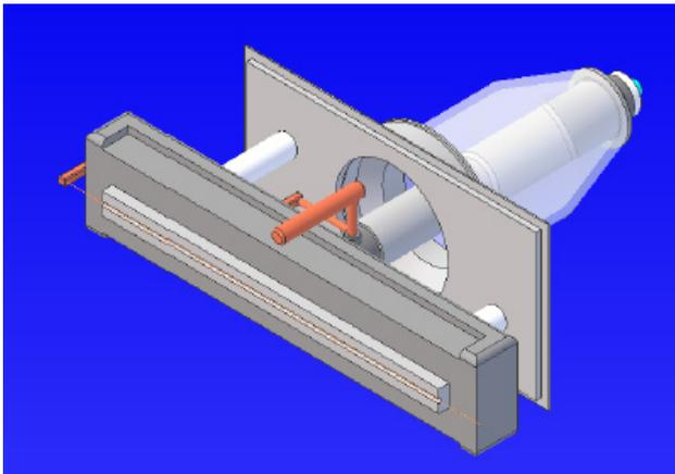
Figure 4: Design of Ribbon strip cathode electron gun.
