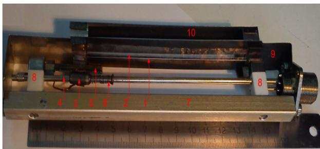
Figure 8: Design of a strip cathode gun with a tension by a spring. 1-filament thorium doped tungsten; 2-slit of extractor electrode; 3-cathode holder, sliding along support rod (4); 4- support rod; 5-plates for direction a cathode holder with a glassy carbon sliders; 6-spring 7-insulated base plate; 8- high voltage insulators;
