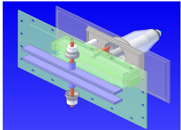
Figure 5: 3D design of RB electron gun with extraction electrode, accelerating anode, and deflection plates.
