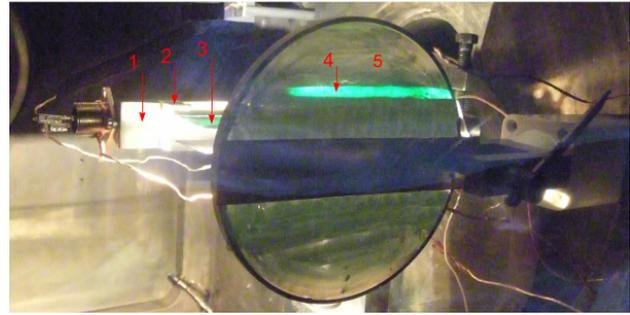
Figure 9: Ribbon electron beam on the luminescent screen deflected by deflection plates. 1-extractor electrode; 2-anode; 3-deflecting plates; 4-image of the ribbon electron beam on the screen; 5-luminescent screen. Diameter of luminescent screen is 110 mm, the shielding plate width is 25 mm.
