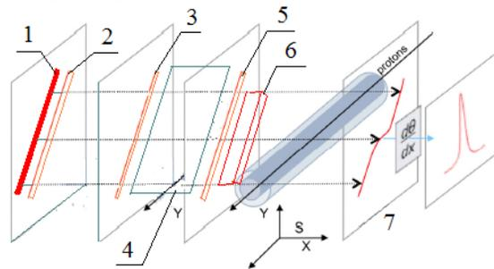
Figure 2: Electron probe beam profile monitor with a strip cathode.
