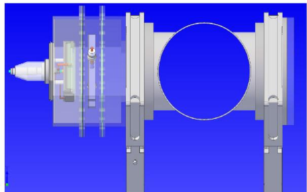
Figure 6: Adaptation of RB e-gun on the vacuum tube of the proton storage ring with vacuum valves.
