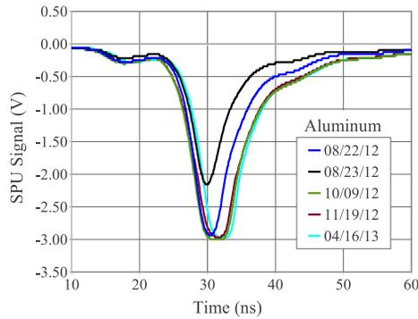
Figure 5: These plots are part of the 2-bunch SPU data in the aluminum chamber at 15E that was taken with 16 mA total positron current (8 mA/bunch =  $1.28 \times 10^{11}$  positrons/bunch). The preamplifier output is limited to 3 V resulting in some flattening of the highest amplitude signals.
