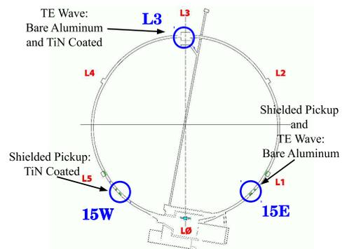
Figure 1: This sketch of the CESRTA storage ring shows the location of detectors used in this study: SPU in a chamber with TiN coating at 15W; SPU and TE wave measurements in the same aluminum chamber at 15E; TE wave measurements in the grooved TiN and bare aluminum chambers of L3.
