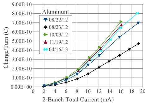
Figure 6: SPU two bunch data from the bare aluminum chamber at 15E shows an overall increase in signal with dose.
