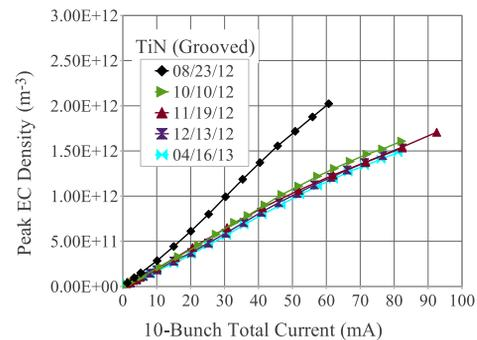
Figure 4: TE wave data with ten bunches from the grooved TiN-coated chamber at L3.
