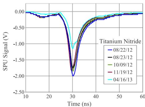
Figure 2: These plots are part of the 2-bunch SPU data that was taken in the TiN-coated chamber at 15W with 16 mA total positron current (8 mA/bunch =  $1.28 \times 10^{11}$  positrons/bunch).
