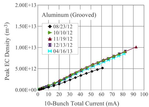
Figure 8: TE wave data from the grooved aluminum chamber in L3 also shows a step increase in EC density after the earliest measurement.
