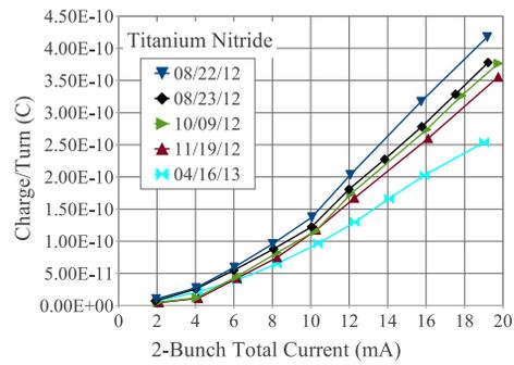
Figure 3: 2-bunch SPU data from the TiN-coated chamber at 15W (see Fig. 2) is integrated to obtain charge/turn. The data shows monotonic conditioning with beam dose. This includes the earliest conditioning with less than 0.5 amp-hours.
