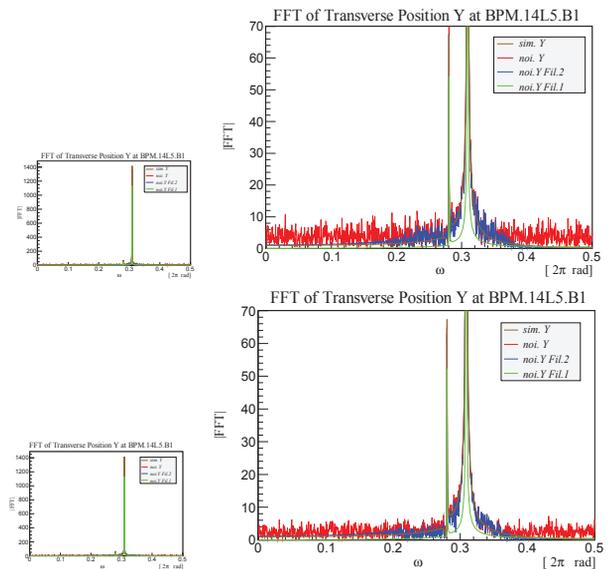
Figure 2: FFT of the Vertical Positions at BPM.14L5.B1 after 2000 turns, with Gaussian (top) and Uniform (bottom) noise. The left plots are the complete spectrum while the right plots is a close-up for the bottom of the spectra. All are a superimpose of a simulated (sim.) trajectory, a sim. with noise added (noi.), and a noise filtered signal for the cases N.1 (Fil. 1) and N.8 (Fil. 2) on Table 1.
