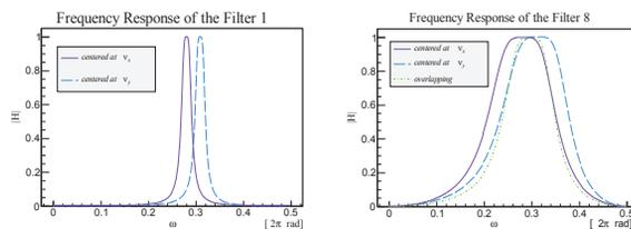
Figure 1: Dual Band-pass filter frequency response, if there is not overlapping (left) and with the corresponding overlapping band (right). Bands centered at 0.2805 and 0.309.
