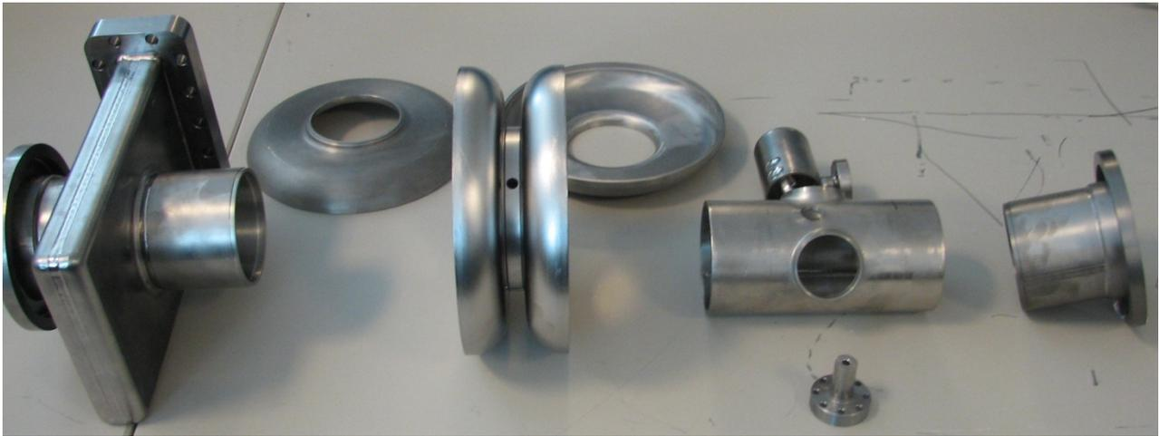
Figure 2: Fabricated 2-cell cavity major components.
