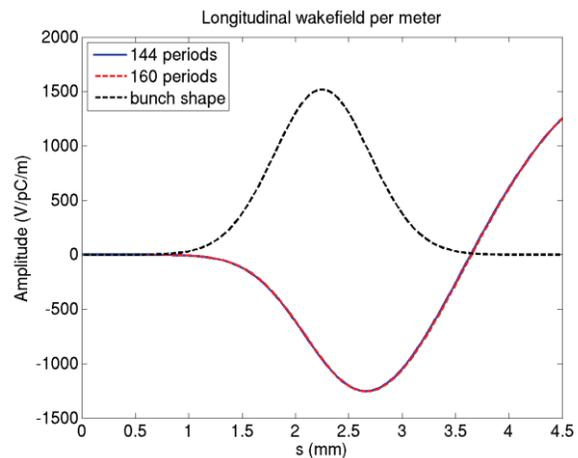
Figure 4: Longitudinal wakefield per unit length of the dechirper with 144 and 166 corrugations.
