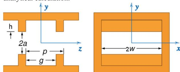
Figure 1: Sketch of the geometry of the dechirper.
