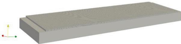
Figure 2: One quarter of the vacuum region of the dechirper model with corrugations situated on a half of the top plate used for T3P simulation. The full model is obtained by reflection with respect to the horizontal and vertical planes.
