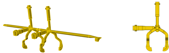
Figure 1: SPX two-cavity deflecting module, and the layout of the FPC and HOM/LOM damping couplers
