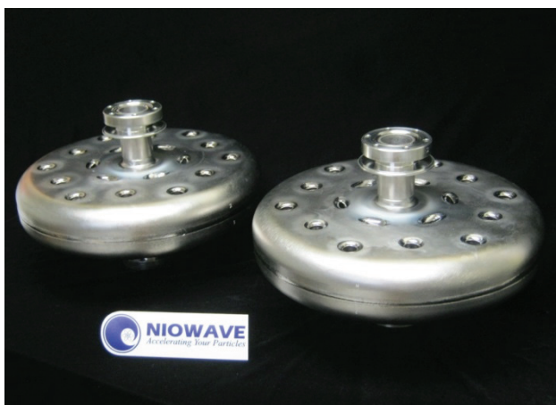
Figure 1: Photograph of the 2.1 GHz PBG cavities with elliptical rods ready to be tested.
